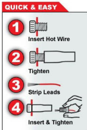
**Scheme 1. How to connect the wires using Posi-taps.**
